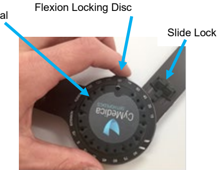
Using the Locking Disc to set Extension Limit at 90°
