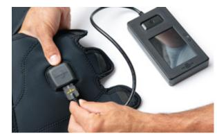
Power on the controller using the ON/OFF switch located on the top left side of the device. The screen will display 2 options:
