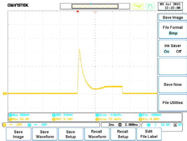
Full output, Voltage across 2,000Ω load
